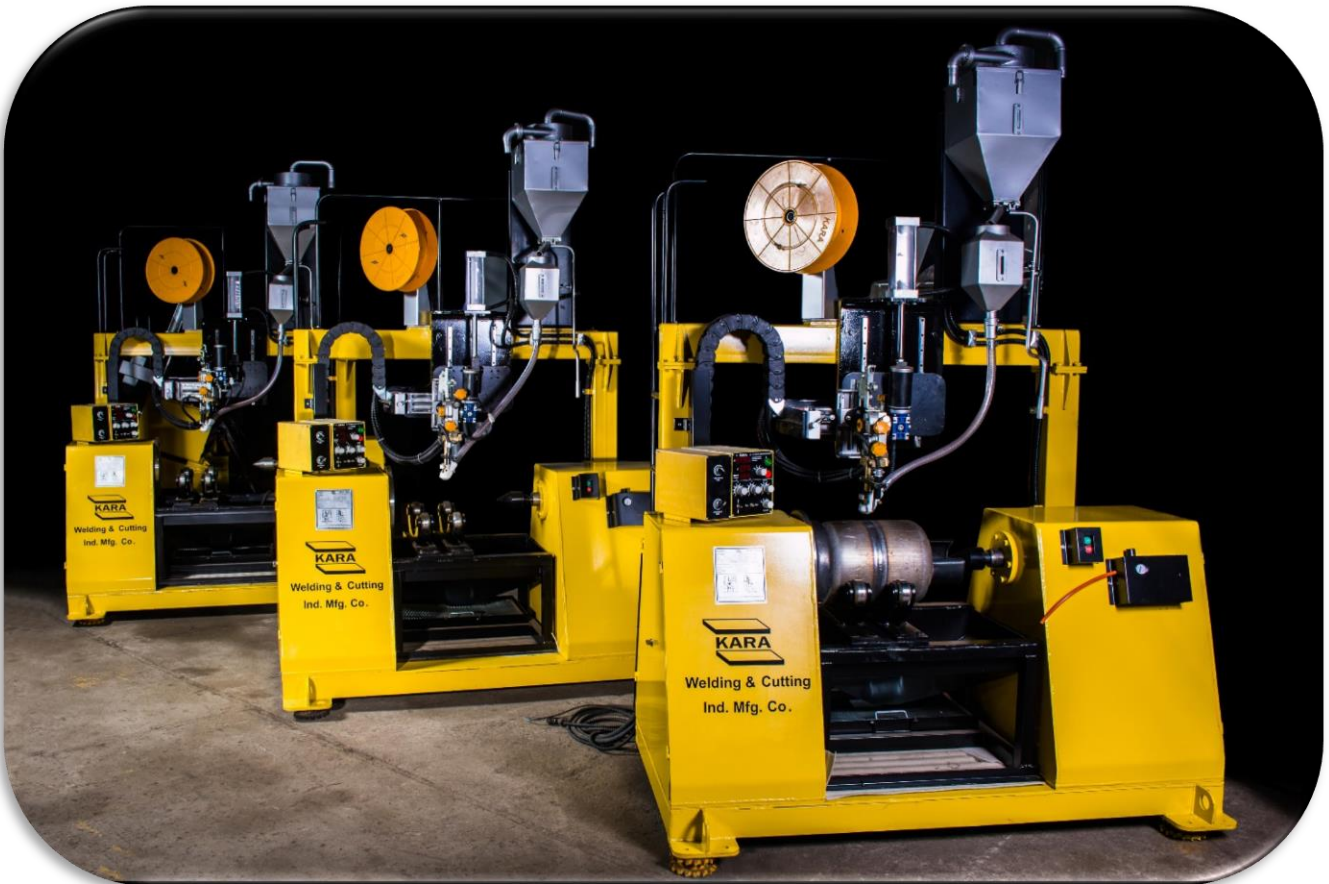
LPG cylinder Circumferential welding machine
